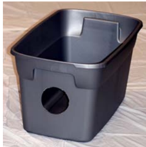
Cut 5 1/2" diameter hole in tote
